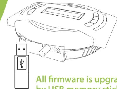
All firmware is upgraded by USB memory stick in a few seconds and no need to disassemble the unit
