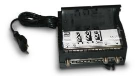
Agile RF converter to process analogue and digital terrestrial channels, able to move a channel from its original frequency to anywhere else in the UHF band (470-862MHz).
