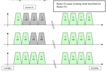
"Mux-ad-Hoc": you can create all the muxes with the choosen programs tuned from up to 8 TV multiplexes and manage all the descriptor parameters of each mux (ONID, TSID, NetID,...) and each program inside the mux (LCN, SID, PID, Program name..).
