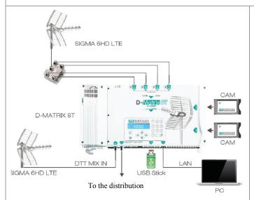
The new D-MATRIX-8T headend can tune up to eight different DVB-T multiplexes, decrypt the programs (through CAMs & Smart-Cards – **NOT INCLUDED**) and generate up to 8 Digital Terrestrial multiplexes (DVB-T), 95dBµV each one.
